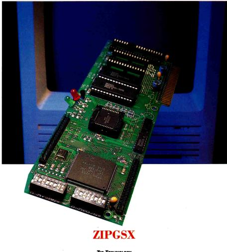
ZIP TECHNOLOGY 5601 West SLAUSON AVENUE, SUITE 190, CULVER CITY, CA 90230, (213) 337-1313 Apple IIGS accelerator card; \$149 (7MHz, 8K), \$199 (8MHz, 16K), \$229 (9MHz, 16K); additional 32K RAM chips, \$49; upgrade to 10MHz, 64K, call for price
